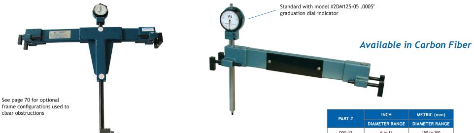
Dorsey Fixed DDG style Depth and Height gages are designed to measure distances from one surface to another. Additionally they can be used to check from a machine fixture to a specific location. The DDG gages are designed for a specific application. Depth units can be used with either a lever transfer or a standard gaging movement. Gaging travel is determined per application.
