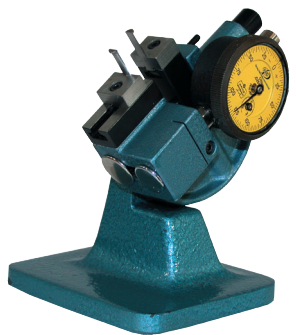
Gage shown is DYS with special metric indicator, part #2305-2 arms part #2349 bench stand
